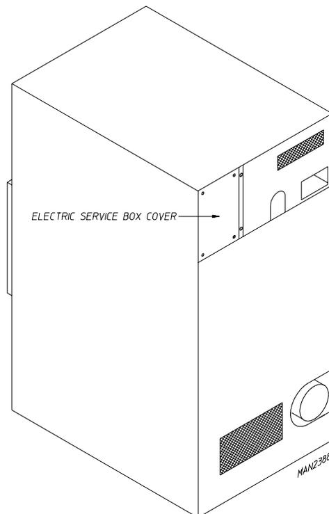
Actual electrical wire connections are made to the L1 and L2 terminals of the motor contactor located in the rear service box mentioned above. The ground connection is also made to the copper lug also provided in this box.
