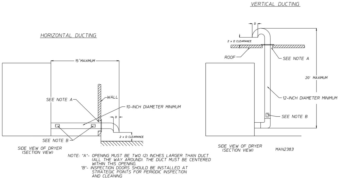
**IMPORTANT:** For extended duct work runs, the cross section area of the duct work can only be increased to an extent. When the duct work approaches the maximum limits noted in this manual, a professional heating venting air conditioning (HVAC) firm **should be** consulted for proper venting information.
