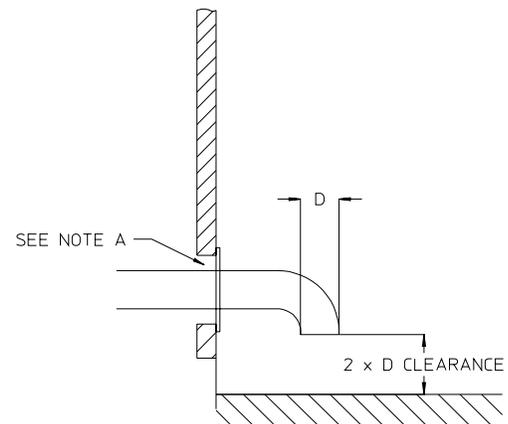
NOTE "A": OPENING MUST BE TWO (2) INCHES LARGER THAN DUCT (ALL THE WAY AROUND). THE DUCT MUST BE CENTERED WITHIN THIS OPENING.
