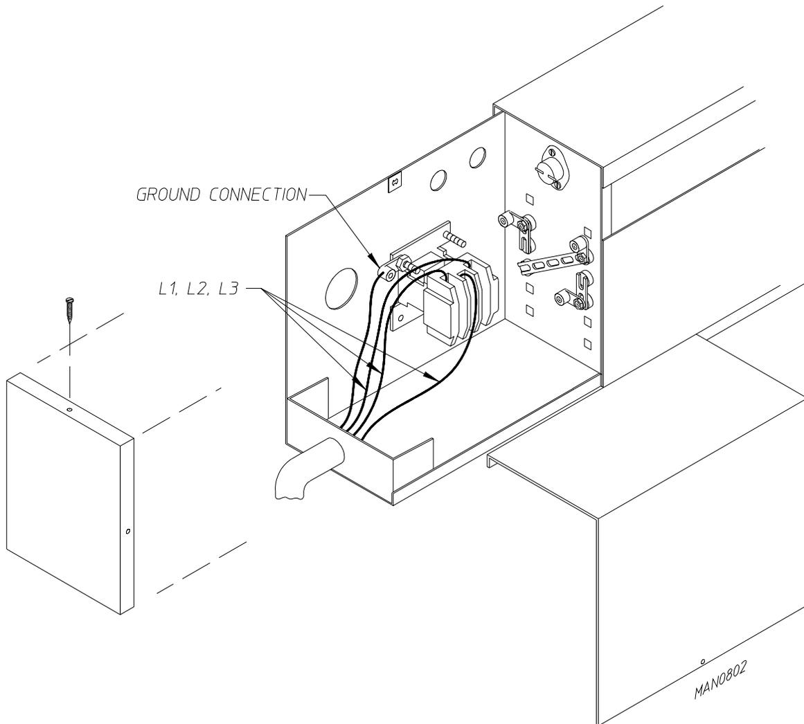
**IMPORTANT:** A strain relief *must be* used where the input wiring enters the oven assembly.
