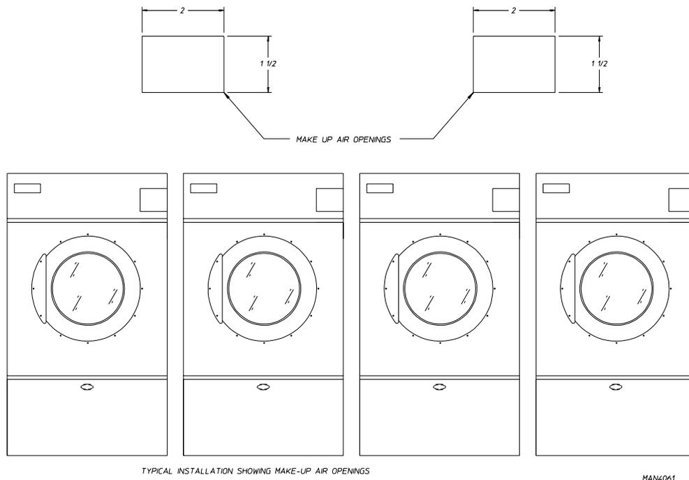
To compensate for the use of registers or louvers used over the openings, this make-up air **must be** increased by approximately thirty-three percent (33%). Make-up air openings **should not be** located in an area directly near where exhaust vents exit the building.
