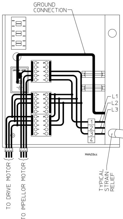
For gas dryers and steam dryers manufactured for operation at 3-phase (3 $\phi$ ), the electrical connections are made at the power distribution block located in the service box at the rear, upper left corner of the dryer. The ground connection is made to the copper lug also provided in this box. To gain access to the service box contactor, the service box cover **must be** removed.
